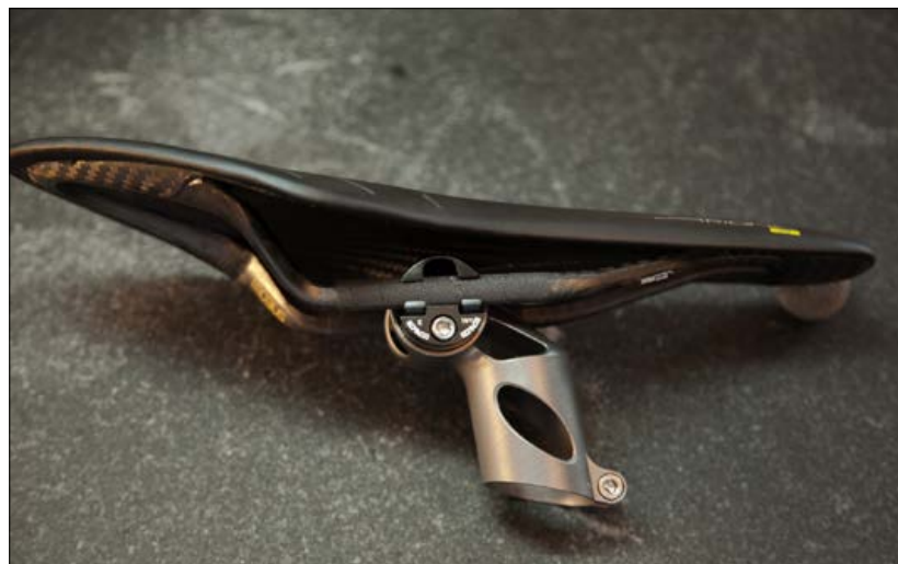
Fig. 1 The completed metal AM titanium seatmast topper with saddle attached (Courtesy Spencer Wright)
