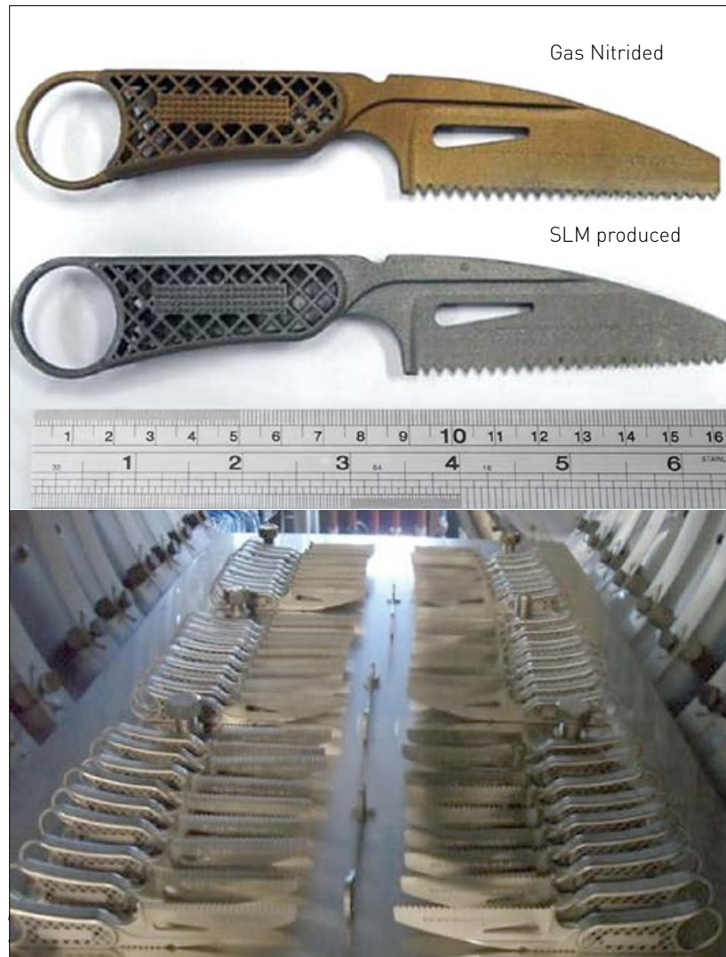
Fig. 11 Gas Nitriding of Ti-6Al-4V knives produced by SLM [3]
