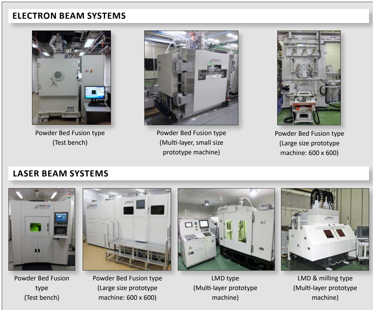
Fig. 11 Electron beam and laser beam systems developed by TRAFAM in 2014, along with two test benches
