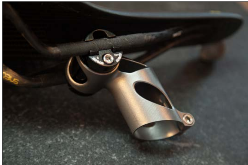
Fig. 10 The part assembled and ready to test (Courtesy Spencer Wright)
