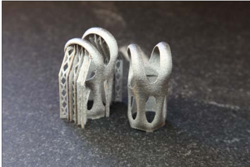
Fig. 13 The new seatpost design, printed in EBM titanium by Addaero (Courtesy Spencer Wright)
