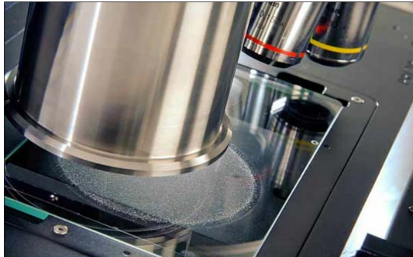
Fig. 3 Shape data for the two samples were collected using the Morphologi G3 from Malvern Instruments
