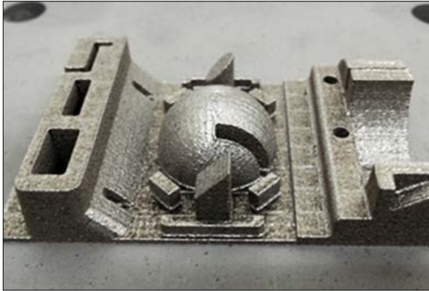
Fig. 12 A trial product manufactured using the TRAFAM Powder Bed Fusion machine
