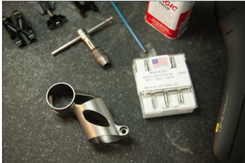
Fig. 9 Preparing to tap the threads (Courtesy Spencer Wright)
