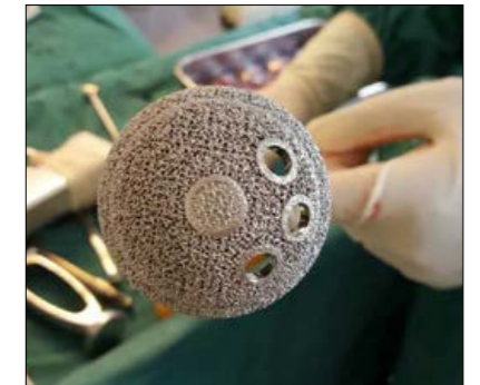
The additively manufactured hip joint has undergone clinical trials
