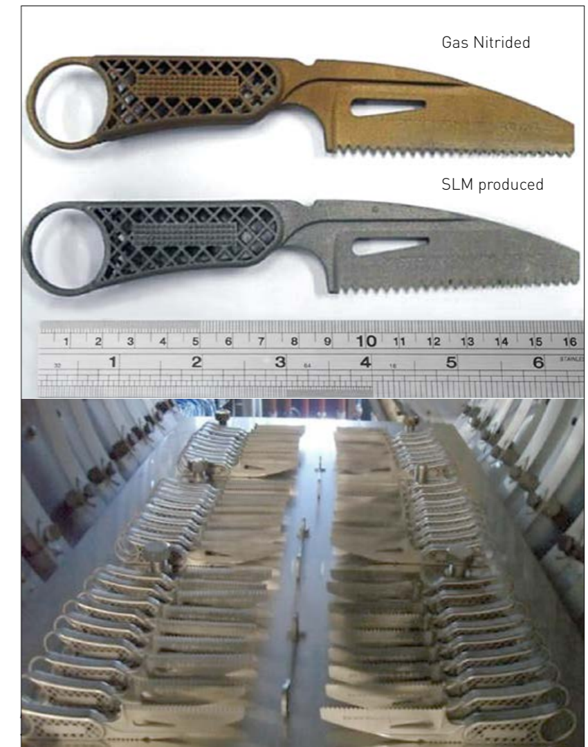
Fig. 11 Gas Nitriding of Ti-6Al-4V knives produced by SLM [3]
