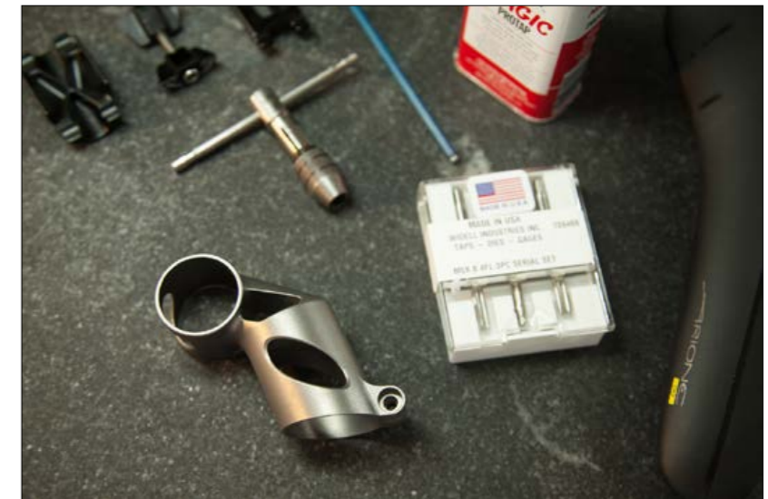
Fig. 9 Preparing to tap the threads (Courtesy Spencer Wright)
