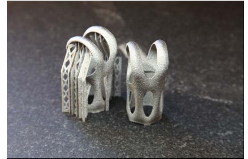
Fig. 13 The new seatpost design, printed in EBM titanium by Addaero (Courtesy Spencer Wright)
