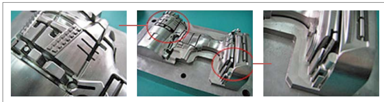
Fig. 7 An example of mould fabricated by a hybrid AM machine (Courtesy of Matsuura Machinery Co.)
