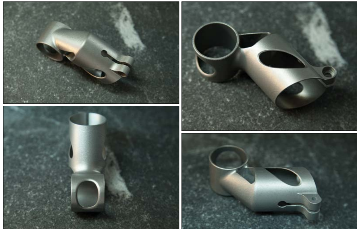
Fig. 8 The second Layerwise build of the part (Courtesy Spencer Wright)
