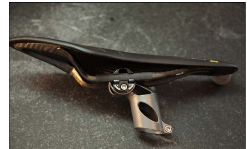
Fig. 1 The completed metal AM titanium seatmast topper with saddle attached (Courtesy Spencer Wright)
