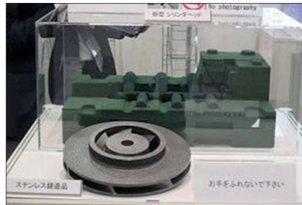
Fig. 14 An example of a casting and a sand mould produced using the TRAFAM prototype machine
