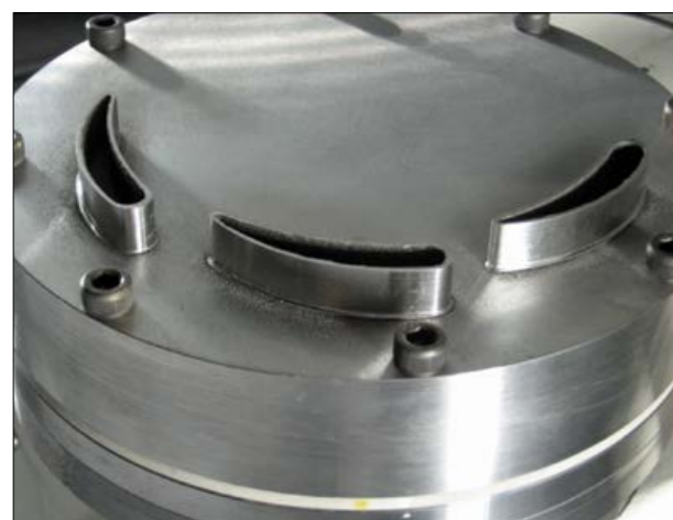
Fig. 13 A trial product manufactured using the TRAFAM Laser Metal Deposition and milling machine
