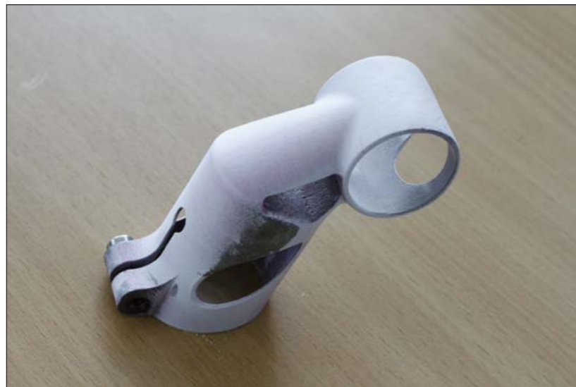
Fig. 12 The part, covered in penetrating dye (Courtesy EFBE)
