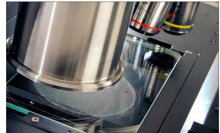
Fig. 3 Shape data for the two samples were collected using the Morphologi G3 from Malvern Instruments
