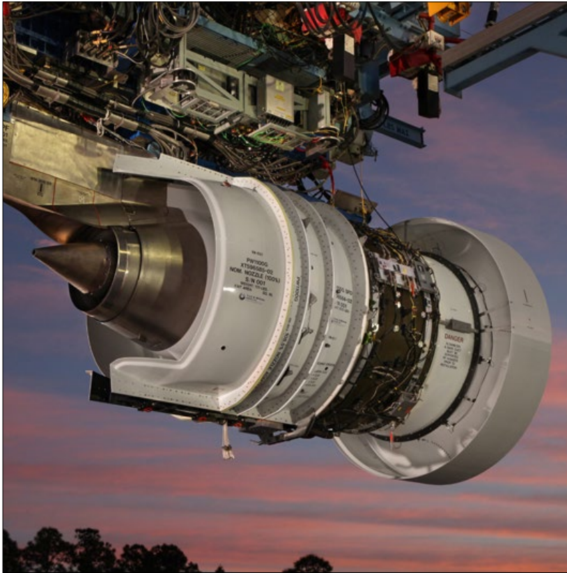
Fig. 2 The first PW1100G-JM engine for the Airbus A320neo during testing on the sea-level outdoor test stand at Pratt & Whitney's West Palm Beach, Florida, facility (Courtesy Pratt & Whitney)
