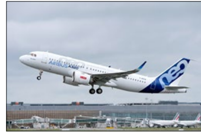
The A320neo Airbus passenger jet is powered by twin LEAP jet engines, each with 19 AM fuel nozzles
