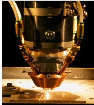
Fig. 4 LENS Engine system in preparation for America Makes Open House [1]
