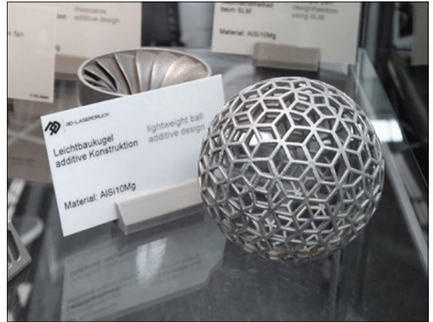
Fig. 3 A lightweight ball design manufactured from AlSi10Mg by 3D-Laserdruck GmbH i.G. (Photo Georg Schlieper)
