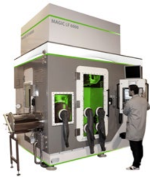
The CLAD MAGIC is a range of machines for AM of metal parts in three and five axis for the aerospace industry
