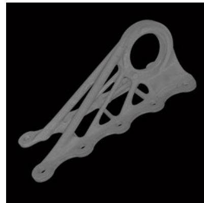
Fig. 4b QMmeltpool 3D display of the cabin bracket from the Airbus A350 XWB with standard output
