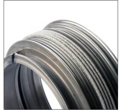
The BeAM Additive Manufacturing machine has been used to repair this worn labyrinth seal
