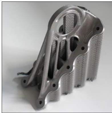
Fig. 5a A cabin bracket from the Airbus A350 XWB with reduced laser output
