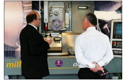
The new millGrind creep-feed grinding machine with integrated laser metal deposition and milling
