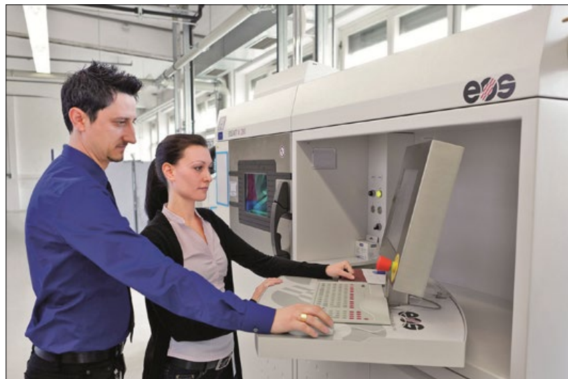
Fig. 4 Manufacturing at MTU: One of the seven EOS systems that produces series components for engine construction (Courtesy MTU Aero Engines)
