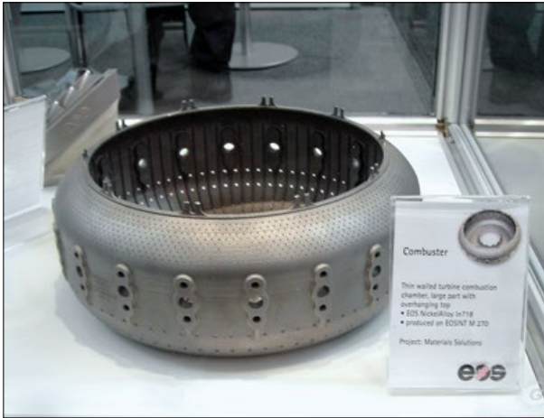
Fig. 2 A thin walled turbine combustion chamber, produced from EOS Nickel Alloy In718 on an EOSINT 270 machine by Materials Solutions (Photo Georg Schlieper)
