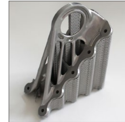
Fig. 4a A cabin bracket from the Airbus A350 XWB with standard output
