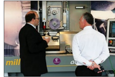
The new millGrind creep-feed grinding machine with integrated laser metal deposition and milling
