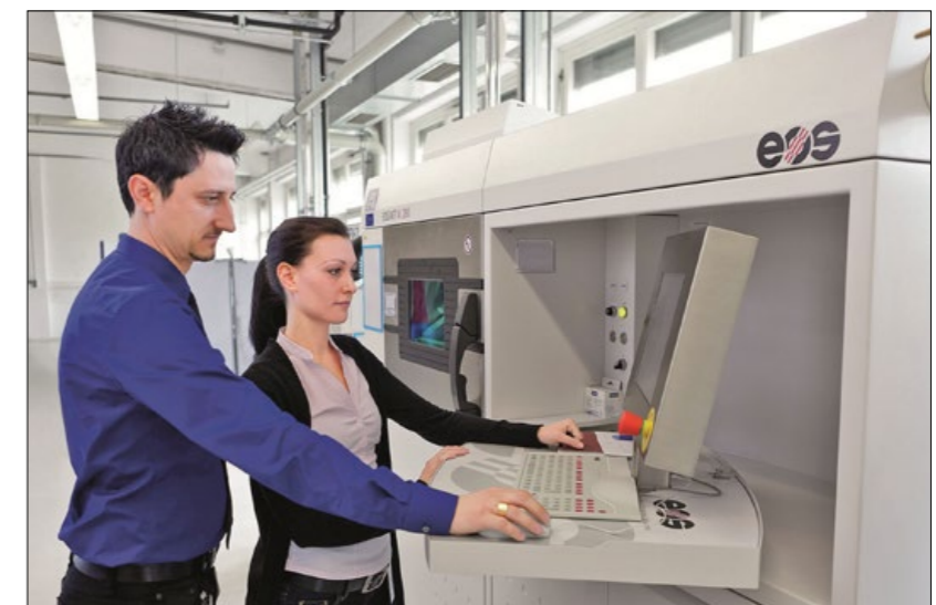
Fig. 4 Manufacturing at MTU: One of the seven EOS systems that produces series components for engine construction (Courtesy MTU Aero Engines)
