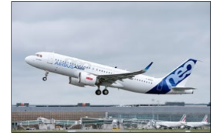
The A320neo Airbus passenger jet is powered by twin LEAP jet engines, each with 19 AM fuel nozzles
