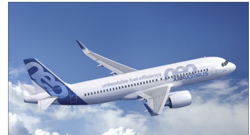
Fig. 1 The Airbus A320neo aircraft features the Pratt & Whitney PurePower PW1100G-JM engine (Courtesy Airbus)
