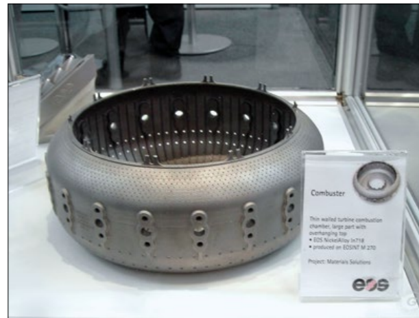
Fig. 2 A thin walled turbine combustion chamber, produced from EOS Nickel Alloy In718 on an EOSINT 270 machine by Materials Solutions (Photo Georg Schlieper)
