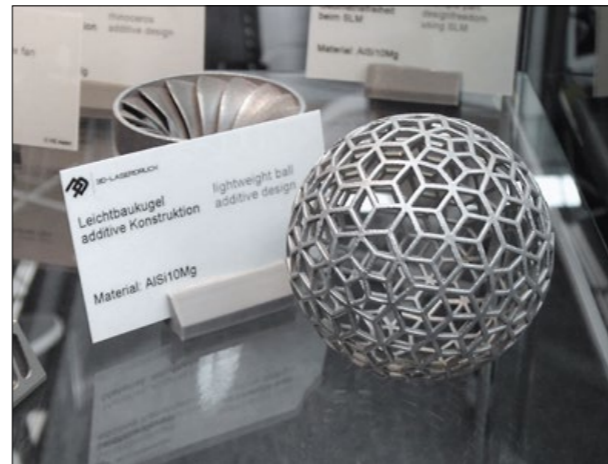
Fig. 3 A lightweight ball design manufactured from AlSi10Mg by 3D-Laserdruck GmbH i.G. (Photo Georg Schlieper)
