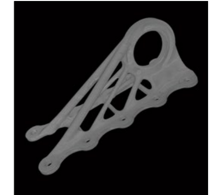
Fig. 4b QMmeltpool 3D display of the cabin bracket from the Airbus A350 XWB with standard output
