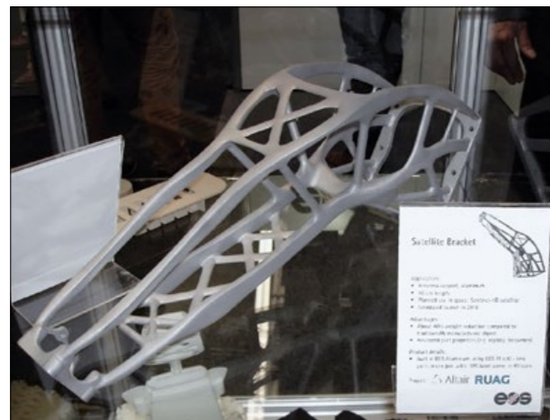
Fig. 4 Additive Manufactured antenna bracket for a Sentinel-1-Satellite, manufactured on an EOS M400 by RUAG Space / Altair (Photo Georg Schlieper)
