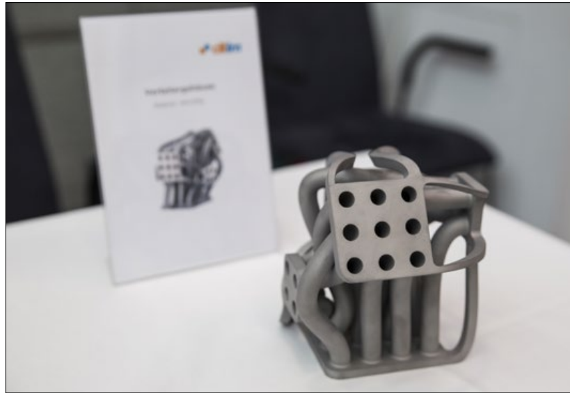
Fig. 12 A number of metal AM parts were displayed at MAMC 2014, including this AlSi10Mg distributor housing manufactured by Citim
