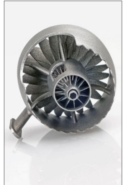
Fig. 4 This model engine production prototype was made in one step, including rotating shaft and 3D wing contours. The AM optimised design was manufactured via LaserCUSING® from stainless steel (1.4404). Minimal reworking thanks to the optimised design. (Courtesy RSC Engineering GmbH)
