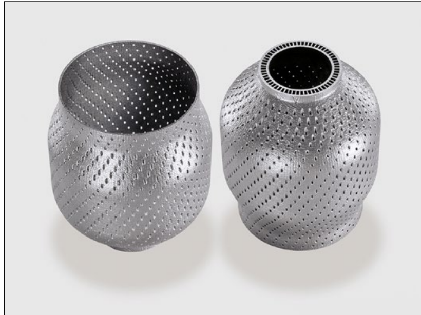
Fig. 5 These models of a cannular combustor have been manufactured to demonstrate the possibility to include effusion holes and a swirler in the manufacturing process (Courtesy Concept Laser GmbH)
