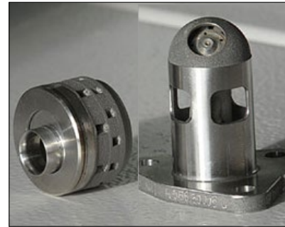
Turbomeca is using Selective Laser Melting (SLM) to manufacture fuel injector nozzles and combustor swirlers
