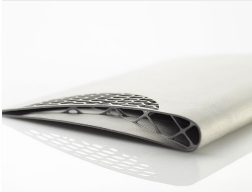
Fig. 3 This model of a wing demonstrates AM's ability to combine differently oriented lightweight structures within one part. The model has been produced in one step (Courtesy Concept Laser GmbH)
