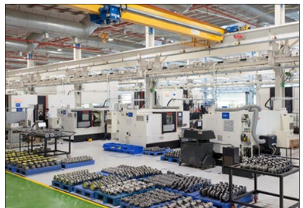
The small parts CNC machining section of the plant (Courtesy Farhad Bomanjee/GE)
