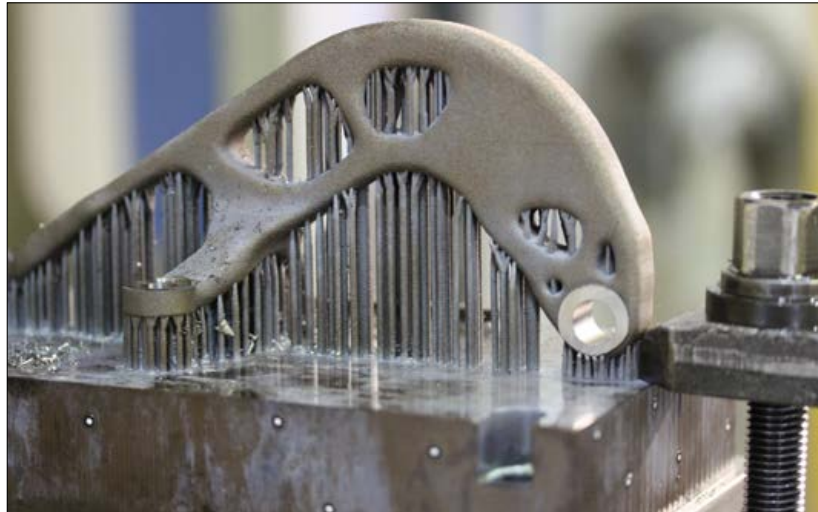
Fig. 31 Here the clamping area for the build plate has been noticeably reduced
