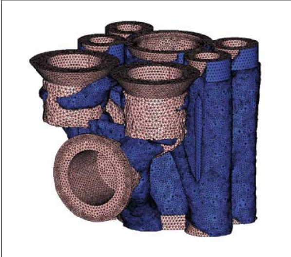
Fig. 2 Generating the valve block shape with OptiStruct
