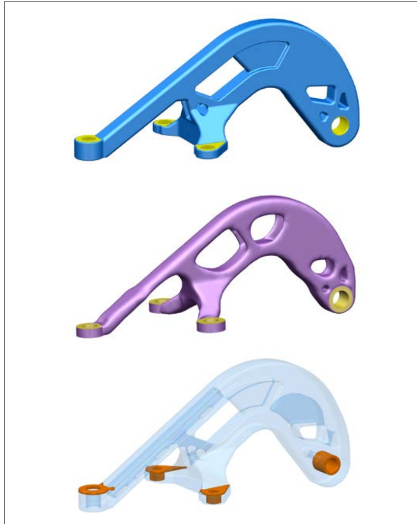
Fig. 7 Net shapes with the surfaces that require machining shown in yellow and additional stock material in orange
