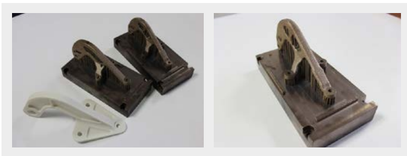
Fig. 18 The brackets after heat treatment with a plastic mock-up of the original part
