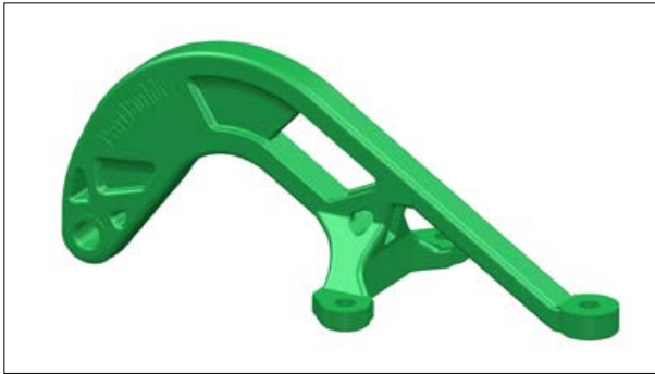
Fig. 13 Design 3, mass optimised with strict manufacturability considerations
