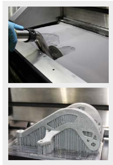
Fig. 17 Manually removing powder with a vacuum cleaner to reveal the parts
