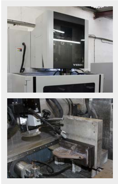
Fig. 22 Wire EDM setup and fixturing: setting up the wire EDM machine by defining part position and alignment before cutting
