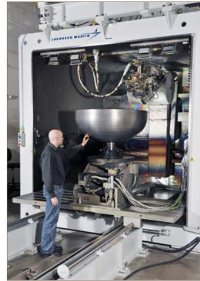
Sciaky has introduced a closed-loop control system for its Electron Beam Additive Manufacturing systems
