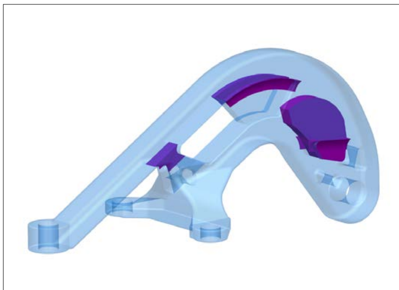
Fig. 12 Design changes to improve manufacturability
