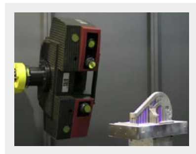
Fig. 19 3D optical scanning
