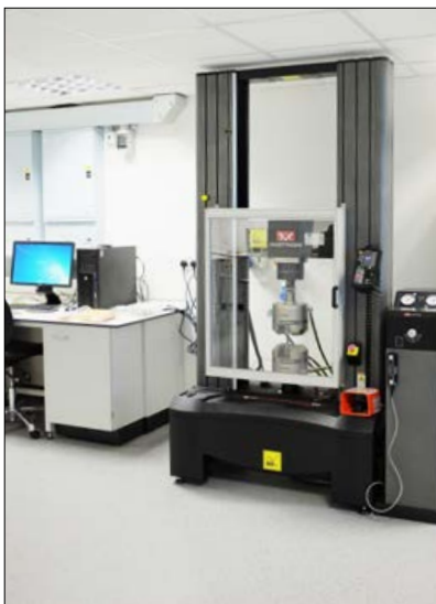
Fig. 3 An Instron tensile testing machine in the laboratory at Renishaw's Stone Solutions Centre
