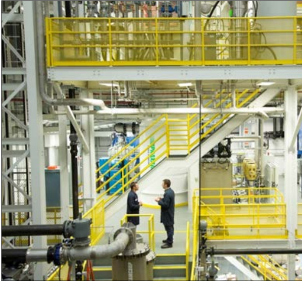
Fig. 2 An atomiser dedicated to titanium alloys at the Praxair Surface Technologies, Inc. powder plant, Indianapolis, Indiana, USA
