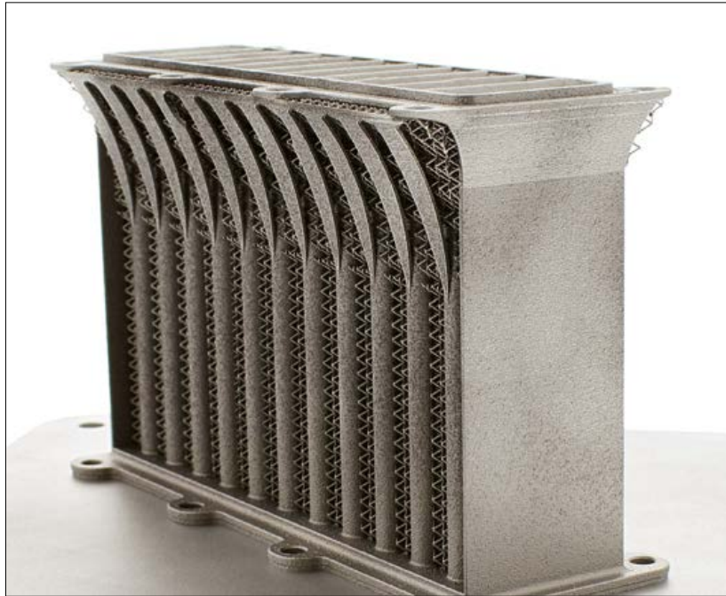
Fig. 9 An intercooler for the Swansea University Formula Student (FSAE) race car, built in aluminium, using Renishaw AM250 system (Image Renishaw plc)
