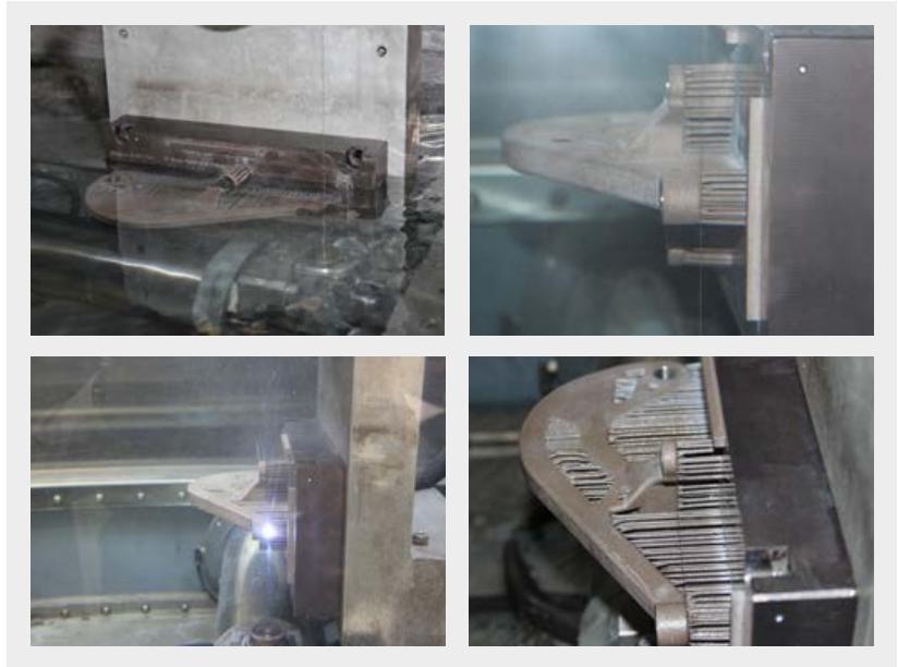
Fig. 23 Wire EDM to separate the part from the baseplate, remove the support fixtures and achieve final part dimensions on some surfaces
