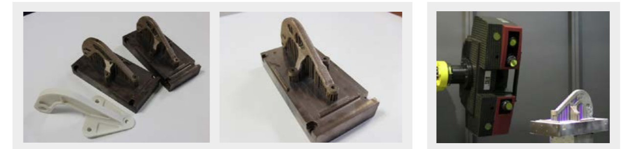
Fig. 18 The brackets after heat treatment with a plastic mock-up of the original part
