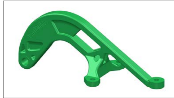
Fig. 13 Design 3, mass optimised with strict manufacturability considerations
