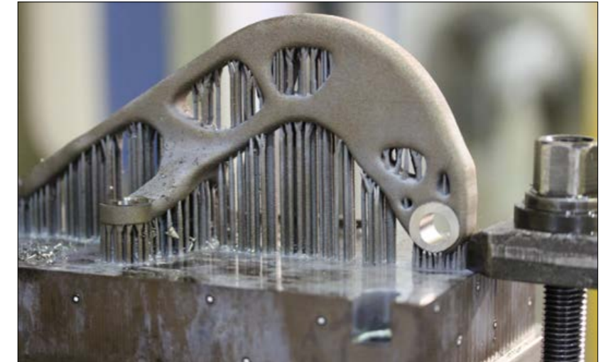
Fig. 31 Here the clamping area for the build plate has been noticeably reduced
