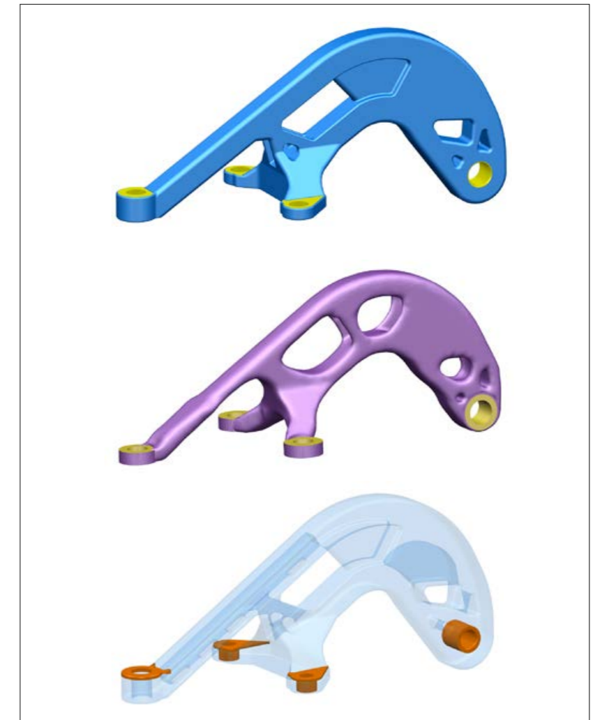
Fig. 7 Net shapes with the surfaces that require machining shown in yellow and additional stock material in orange
