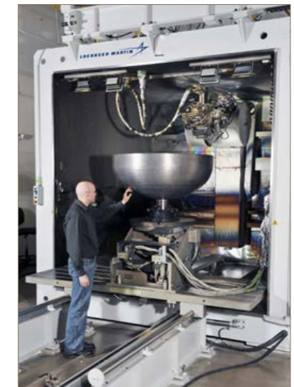
Sciaky has introduced a closed-loop control system for its Electron Beam Additive Manufacturing systems
