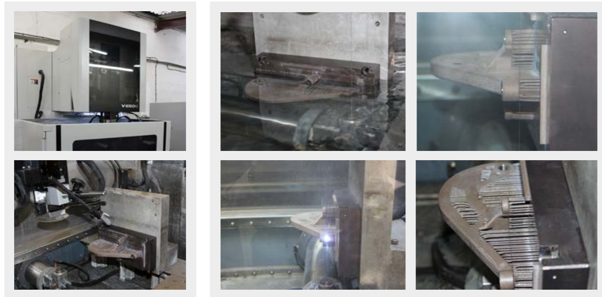
Fig. 22 Wire EDM setup and fixturing: setting up the wire EDM machine by defining part position and alignment before cutting
